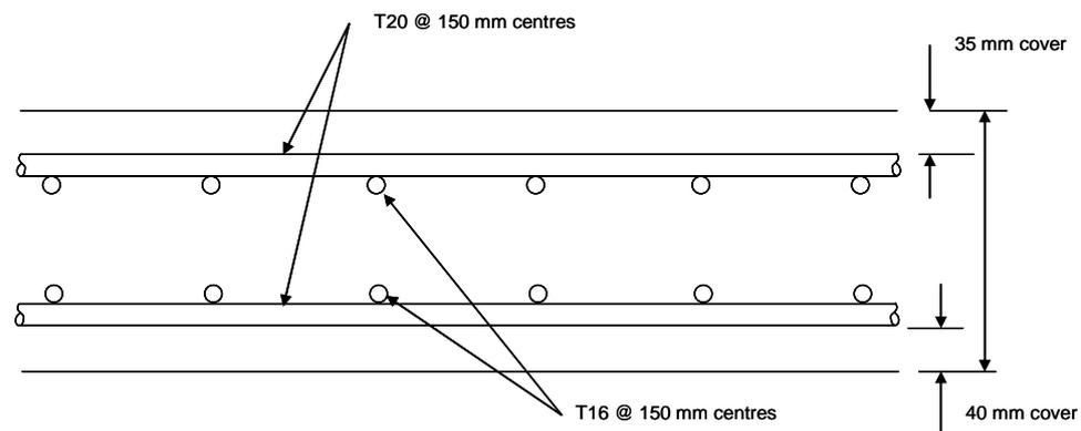
Figure 8.2 Slab reinforcement
