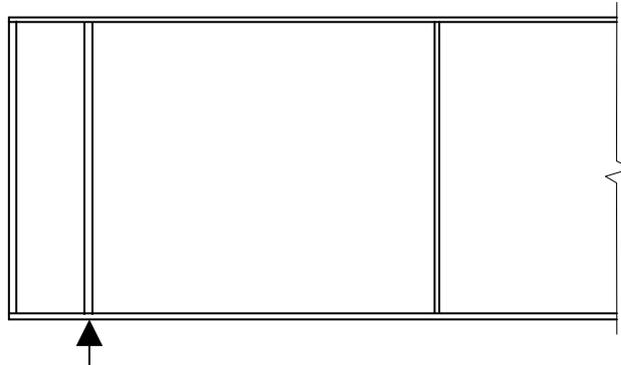
**Figure 7.3** End post detail at an end support
