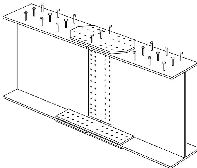
Figure 14.1 Girder splice, showing cover plates and shear studs
