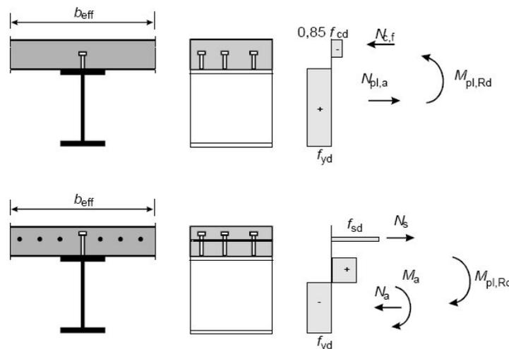
**Figure 5.1** *Plastic stress distributions in a composite beam*
