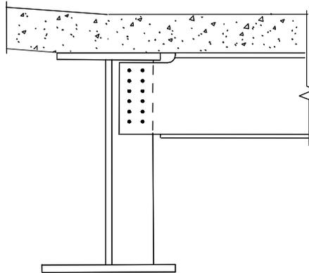
**Figure 14.2** Connection of intermediate cross girder in a ladder deck bridge
