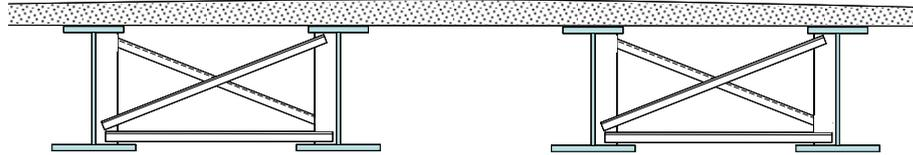
Figure 6.2 *Bracing between paired beams*
