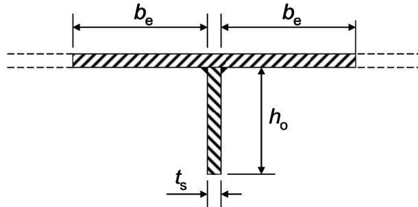
Figure 11.1 Effective stiffener section
