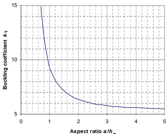
**Figure 7.1** Shear buckling coefficient  $k_\tau$
