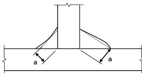
**Figure 13.1** *Effective throat of a fillet weld*
