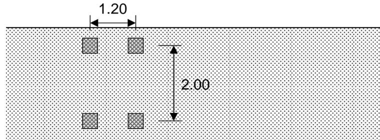
**Figure 2.1** Load Model 1- arrangement of Tandem System within loaded lane
