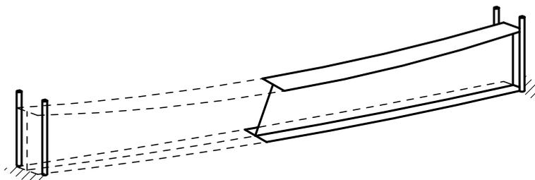
**Figure 8.1** *Lateral torsional buckling of a simply supported beam*
