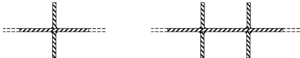
Figure 12.1 Bearing stiffener arrangements
