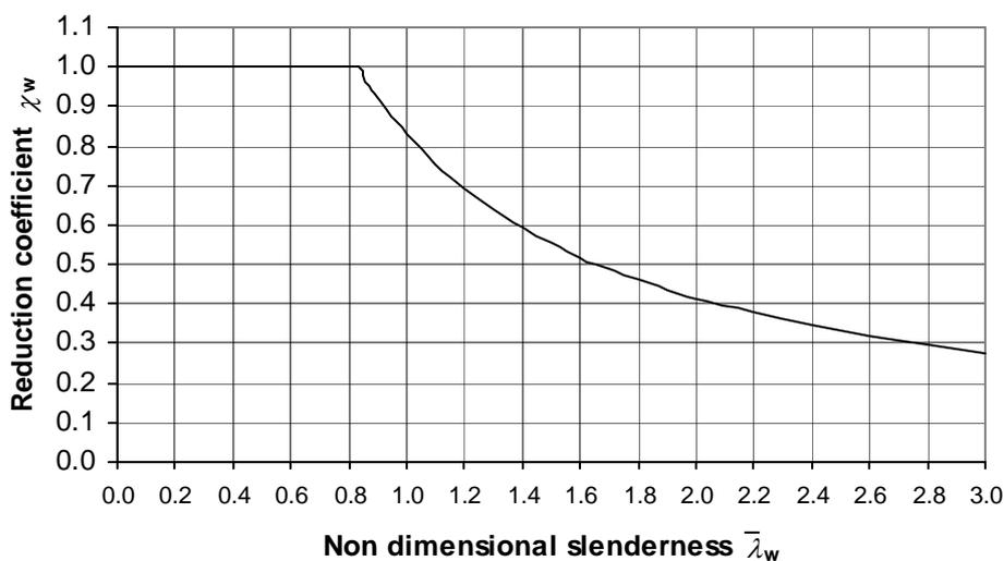
**Figure 7.2** Shear reduction factor  $\chi_w$
