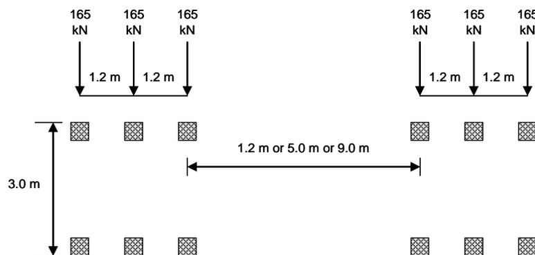
**Figure 2.2** Load Model 3 vehicle
