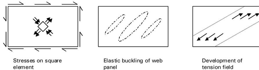
**Figure 7.4** *Web Panels in shear: buckling and tension field action*
