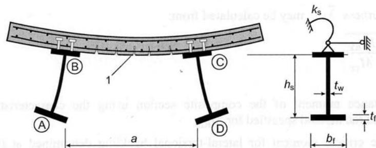
**Figure 6.1** *Distortional buckling*
