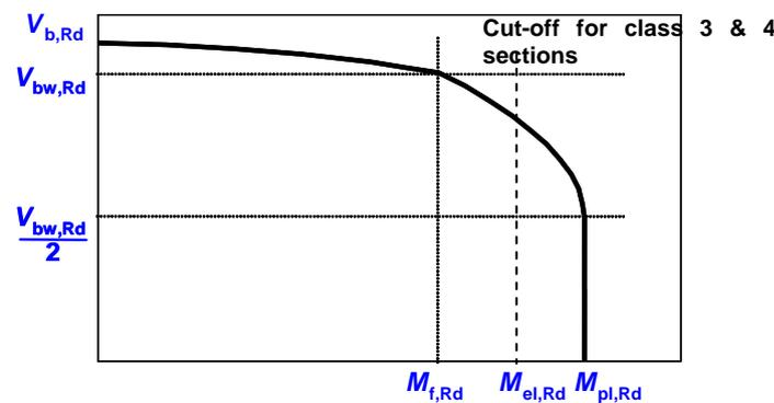
**Figure 7.5** *Limiting interaction between moment and shear resistances*
