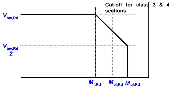
**Figure 7.6** Simplified interaction diagram
