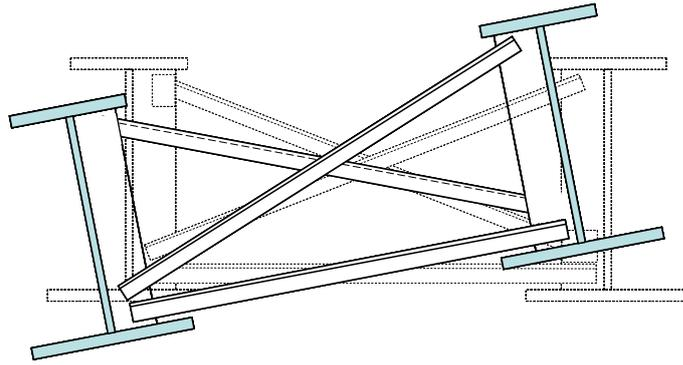
**Figure 10.1** *Buckling mode for paired beams - torsional restraints*
